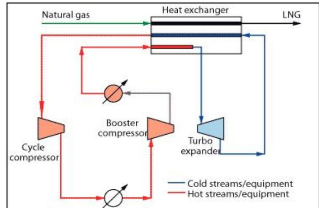
Figure 1 – The Nitrogen Expander Cycle
