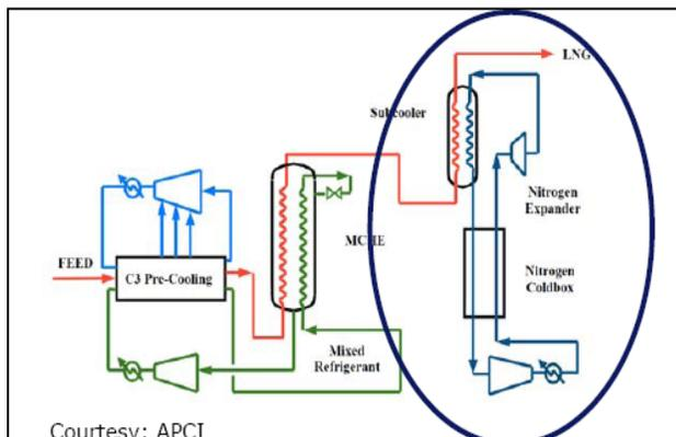
**Figure 2 – Large scale reference for the Nitrogen Expander Cycle**
