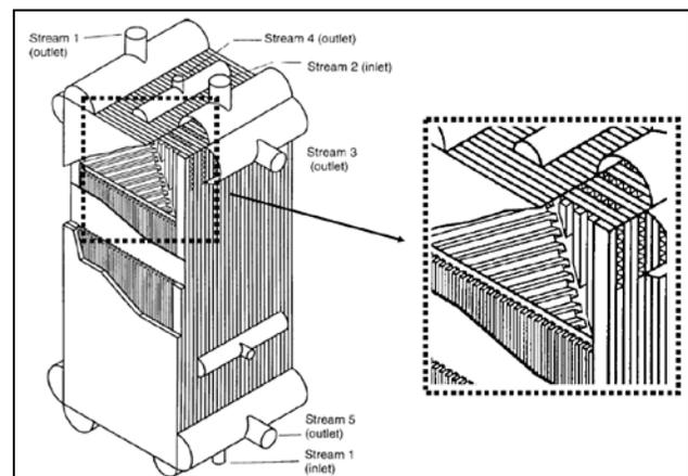
Figure 4 – Illustration of a typical multi-stream brazed aluminium plate-fin heat exchanger
