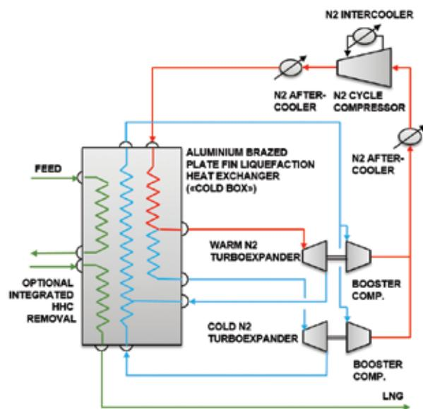
**Figure 4.** Aragon's Optimised Dual N<sub>2</sub> Expander Cycle.
