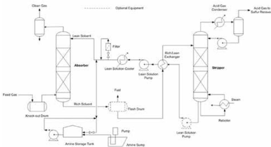
**Figure 2.** Typical process scheme regenerative absorption process.
