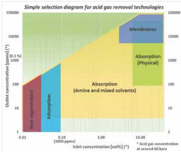
**Figure 1.** Technology selection for sour gas (CO<sub>2</sub>) removal.
