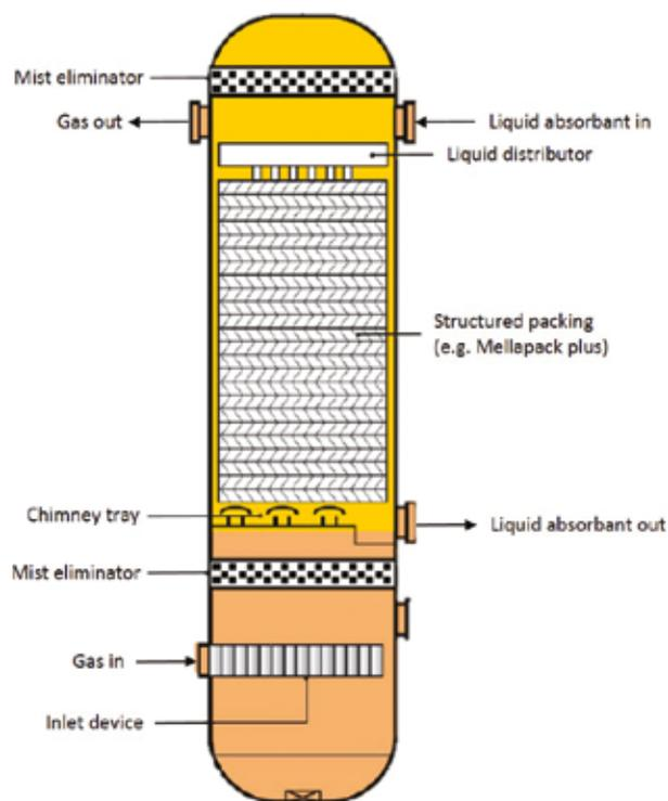
**Figure 3.** Simplified view of column internals. (Column drawing by Sulzer.)
