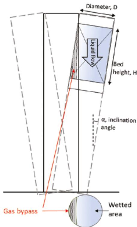
**Figure 4.** Packing maldistribution and non-wetted sections.
