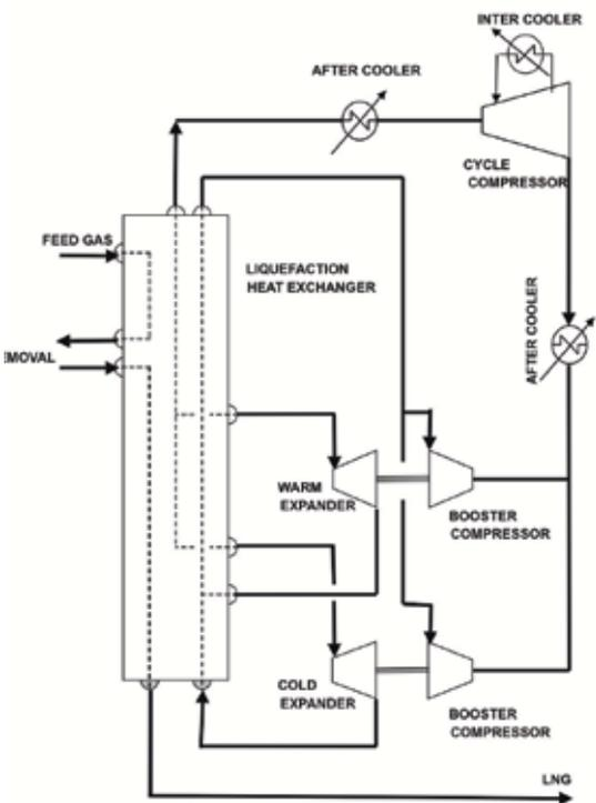
Figure 2. A typical nitrogen expander cycle.
