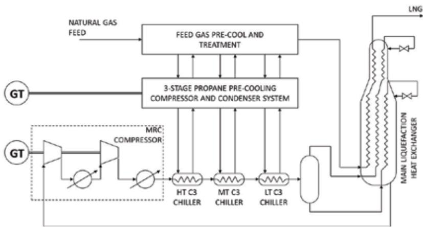
Figure 1. A typical mixed refrigerant cycle.
