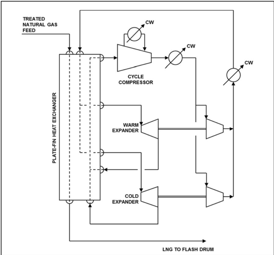
Figure 1 Typical flow scheme of a dual nitrogen expander cycle.
