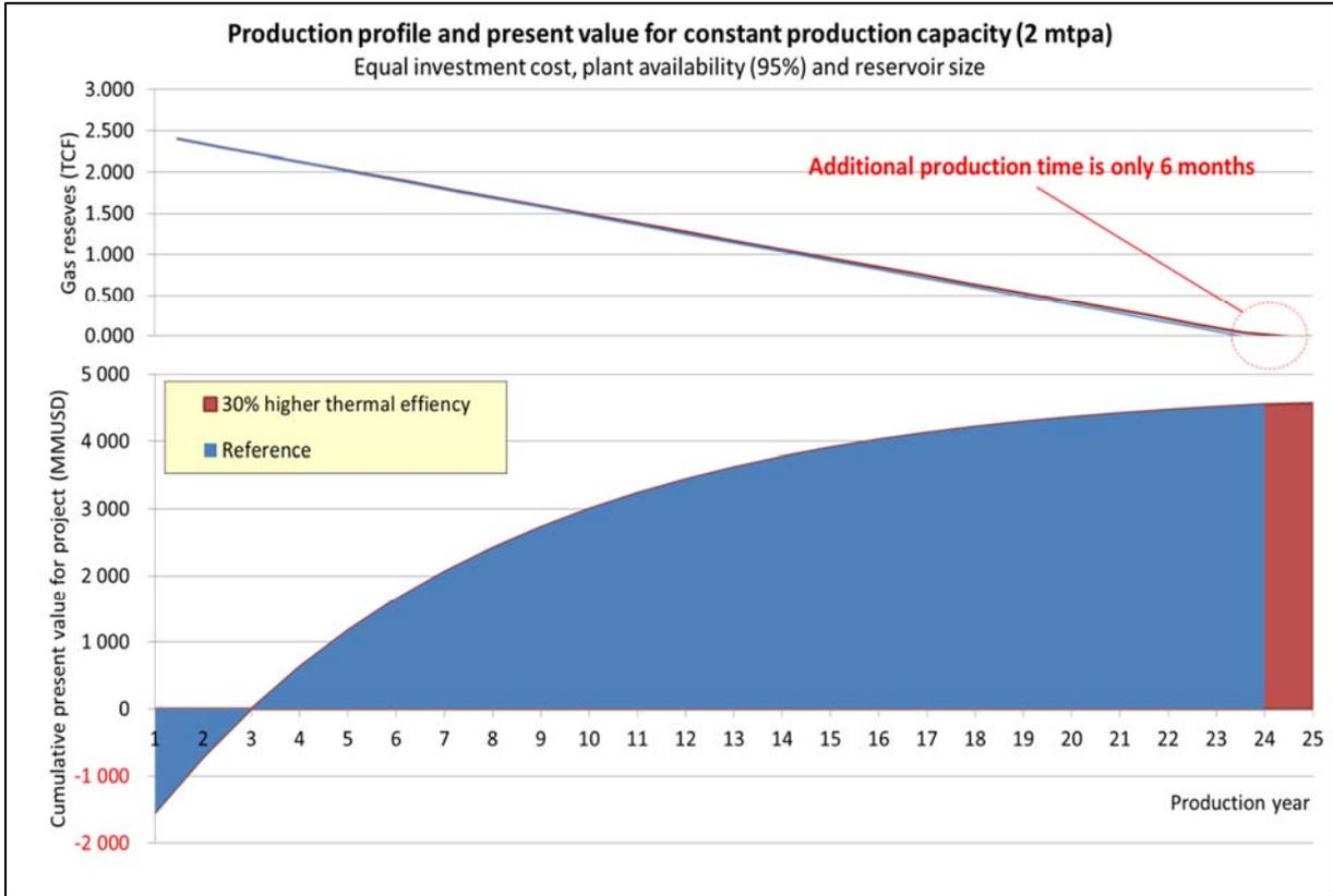
Figure 4 Production profile and present value for constant production capacity.
