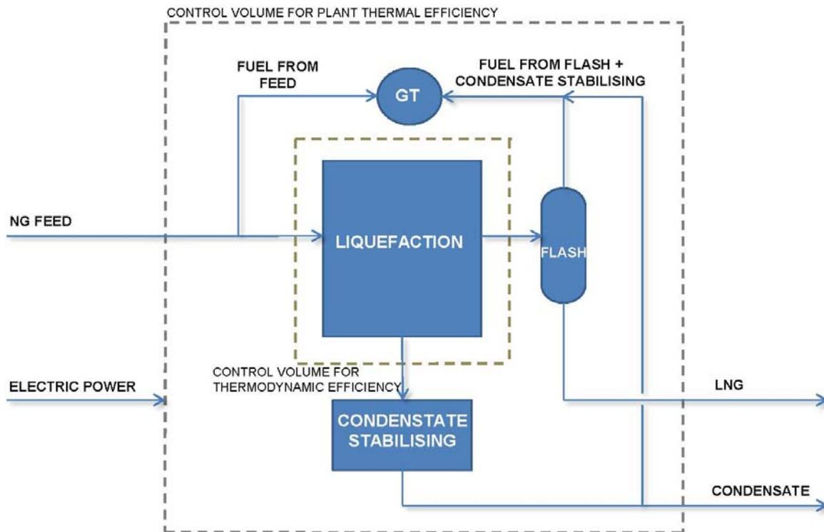
Figure 3 Figure demonstrating theory behind thermal and thermodynamic efficiency calculation.
