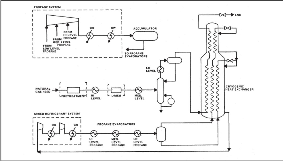
Figure 2 Typical flow scheme of a propane pre-cooled mixed refrigerant process [1].
